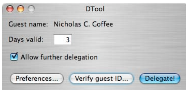
Figure 1: A screenshot of our delegator tool (a trusted Java applet, shown running under Mac OS 10.3). Before delegation, the delegator has to verify the identity of the guest’s public key using a visual hash comparison. Also notice the inputs for validity interval and whether or not to allow further delegation.
